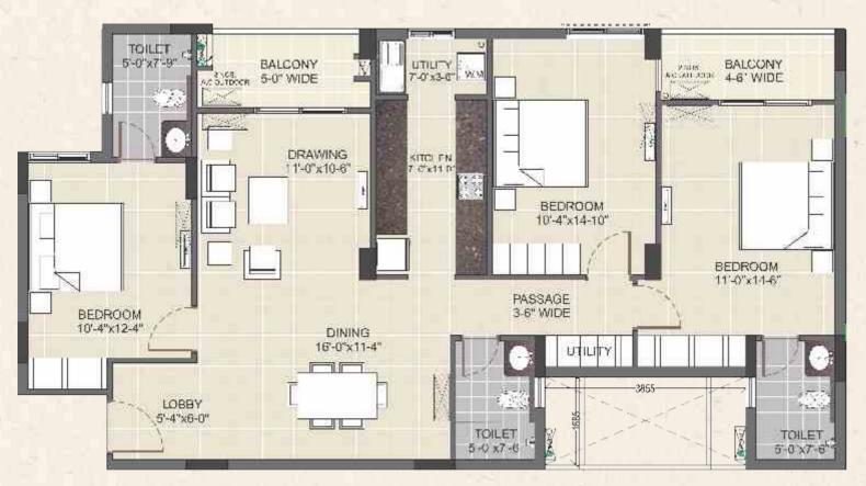
• The Internal Dimensions shown are from wall to wall excluding plaster thickness as per Architectural & Structural construction drawings.
